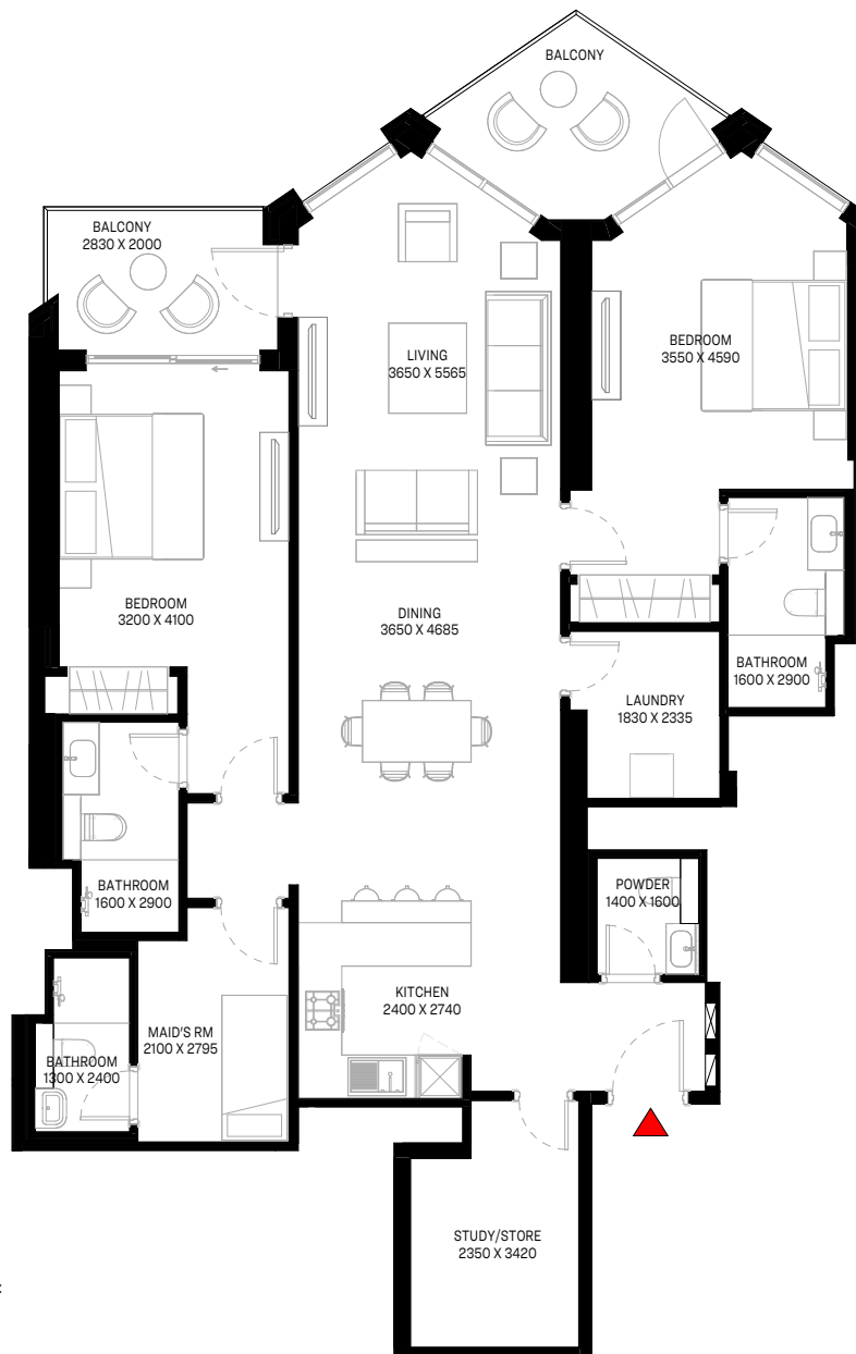
TYPICAL FLOOR PLAN (10,12,14,16,18,22,24,26,28,30,32)_LOWER LEVEL
